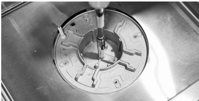
Loosen and remove the NG ORIFICE
